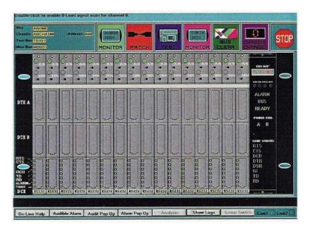
In this example the DCC displays an EAS A/B chassis front panel. The status of each channel's interface is displayed continuously, as is the A or B fallback position. A drag and drop menu on the top of the screen allows the user to sue the integral buses for monitoring or testing any circuit. The patch icon allows for an electronic patch. Double click on the DCE port to view the full interface and alarm status.
